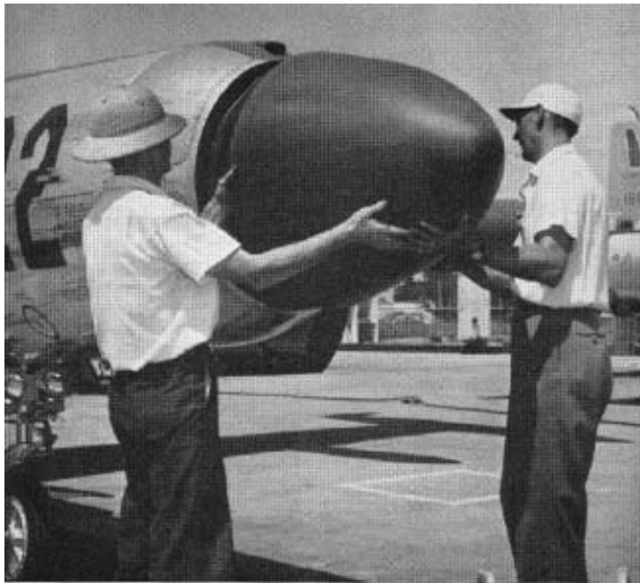
FIG. 2 GLASS REINFORCED PLASTIC RADOMES, INSTALLATION. MONSANTO MAGAZINE, JULY 1954.
