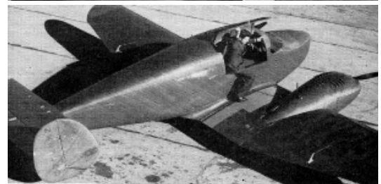
The finished product. Langley's all-molded plywood ship passed preliminary tests last year. Designed as a "family plane," it may become a bomber trainer.
